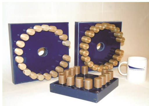
Figure 5. PowerMod™ high-voltage solid-state switch modules. The larger switches consist of 20 IGBTs in series and are rated for 10 kVDC at 100 A peak current.
