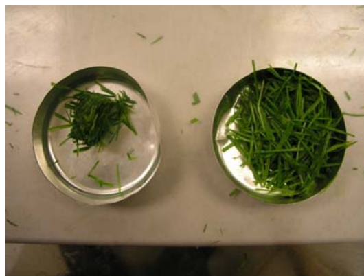
Figure 6. PEF treated (left) and untreated (right) wheatgrass samples. Although the raw masses are identical for each sample, the PEF treated sample appears wilted and wetter. More than 30% more liquid was
