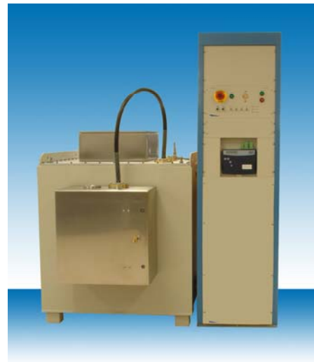
Figure 1. Commercial PEF System for wastewater treatment. This system is rated at 35 kV, 350 A peak pulses, and delivers 150 kW of average power. The modulator is on the left, with the treatment chamber in the 'sidecar' box shown in front. The rack on the right contains the controls and data logging system.
