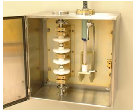
Figure 2. Commercial co-field flow treatment chamber, shown inside the 'sidecar', with four treatment cells. Pipe diameter is approximately 1.5 cm.
