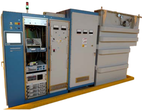
DTI Hybrid System. This ESS-class klystron test stand leverages a solid-state driven pulse transformers to provide a stable high voltage pulse (115 kV) over 3.5 ms.
