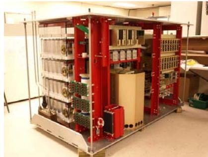
Fig. 6. Long pulse ILC Marx modulator in final stages of completion at DTI.
