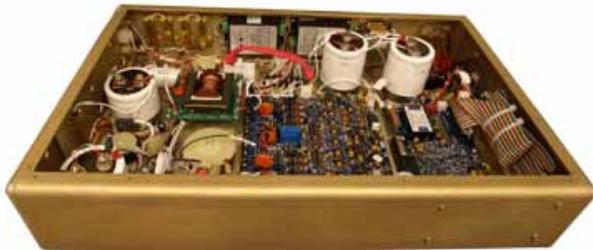
Figure 4. Floating supplies for the heater, grid, and ion pump.
