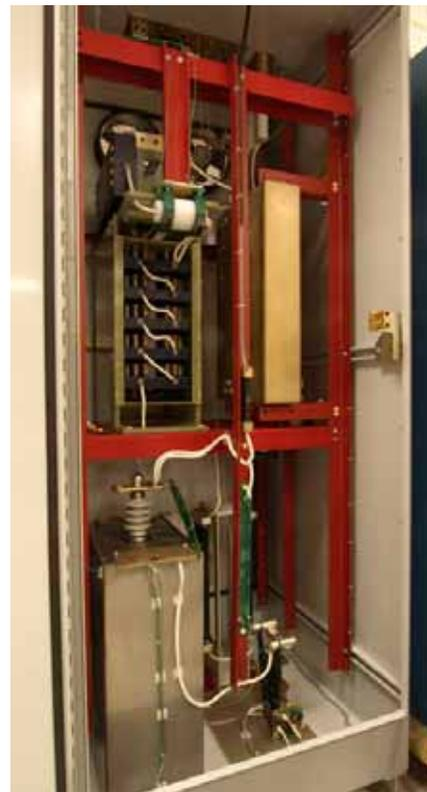
Figure 3. High-voltage cabinet for the pulsed amplifier. The modulator is at the middle left, and has blue switch plates. This cabinet is air-insulated.
