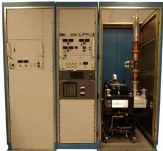
Figure 1. Modular multiple-frequency RF amplifier, CW version. The left cabinet holds the inverter, controls and tank for the HV power supply (behind a panel). The middle cabinet holds the solenoid supply, control box for faults and auxiliary supplies, RF metering, RF predriver, and RF driver. The right rack contains a 704 MHz IOT and cavity.
