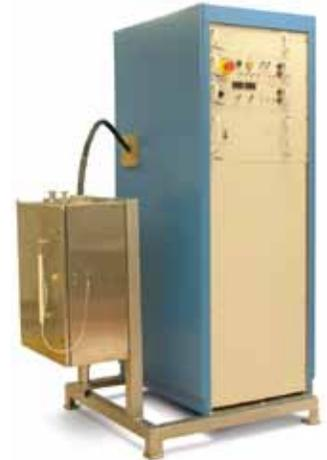
**PEF pilot plant** with a capacity of up to 400 liters/hour. The power supply, modulator, and controls are in the cabinet on the right. Treatment chambers are in the enclosure on the left.
