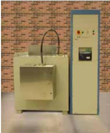
**PEF wastewater treatment system** comprised of a DC power supply rated at 150 kW, a 40 kV, 500 A pulse modulator, and a treatment chamber with four, 15 mm treatment gaps. It processes 10,000 liters/hour of wastewater sludge prior to anaerobic digestion.
