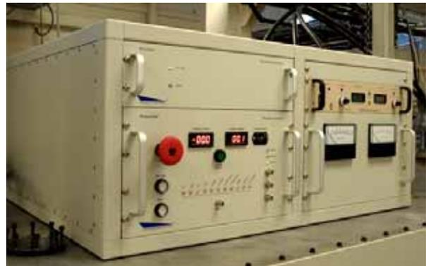
**Figure 6.** Modulator Controls, including fast fault detection and first fault identification.
