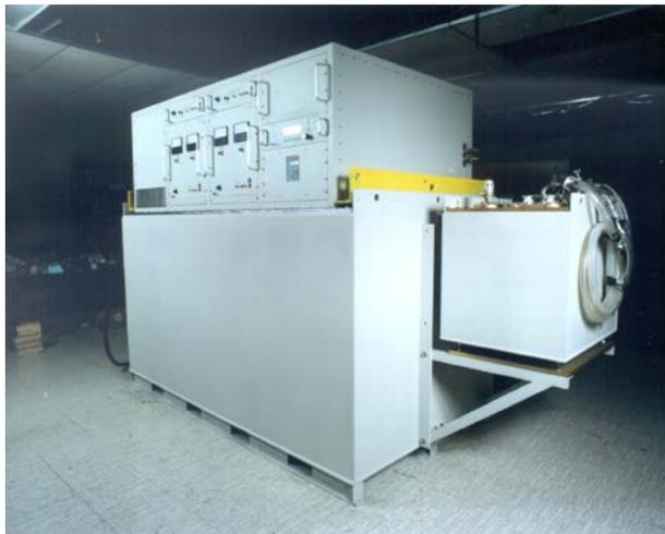
**DTI built the world's first commercial scale PEF food processing system**, based upon DTI's PowerMod™ electronics, in association with Ohio State University's department of Food Science and Technology.
