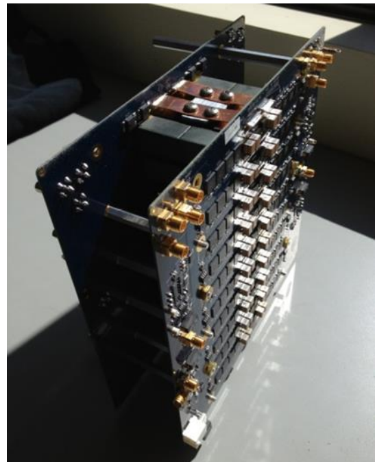
Fig. 1. Dual PCB high speed pulser kicker driver system developed by DTI for the NGLS program. This kicker uses commodity 650 V transistors to switch nearly 17 MW, 700 A in 5 ns.
