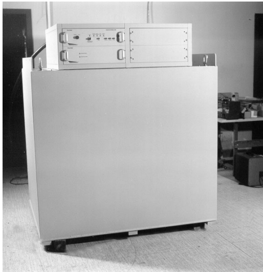
Figure 4: PowerMod™ 70 MW modulator
